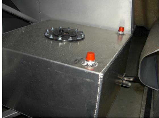
1 of 2 fuel cells to be installed
