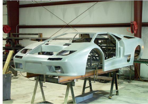
Body being mounted on chassis
