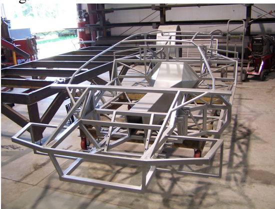
Tubular chassis before suspension
